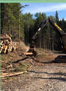
During the site visit to a cutblock, a harvester calibration was performed to ensure products met block specifications. This type of testing is performed on a regular basis to ensure merchantable products are maximized while minimizing waste.
